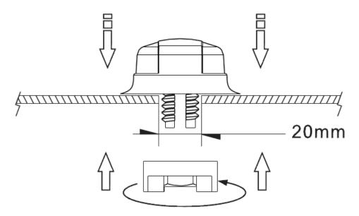
◎Recommended torque setting for mounting is 95 Nm. or 70 ft. Ibs
