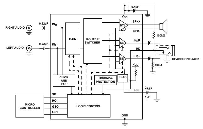
ISL54004 Typical Application Circuit and Block Diagram
