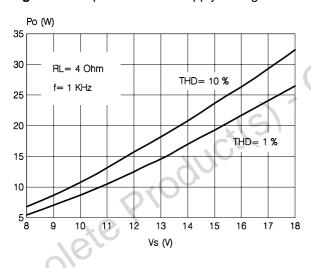
Figure 6: Distortion vs. Output Power
