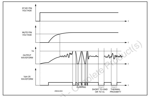
Figure 14: Diagnostics Waveforms.
