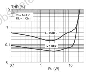
Figure 7: Distortion vs. Frequency.
